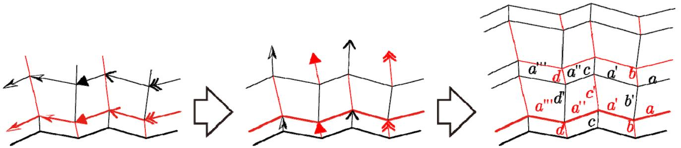
Fig. 8: Construction of planar tessellation with rigid-foldability.
