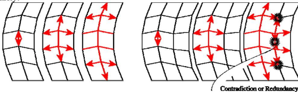
Fig. 4: One-DOF foldable mechanism (left) vs. over constrained mechanism (right).
