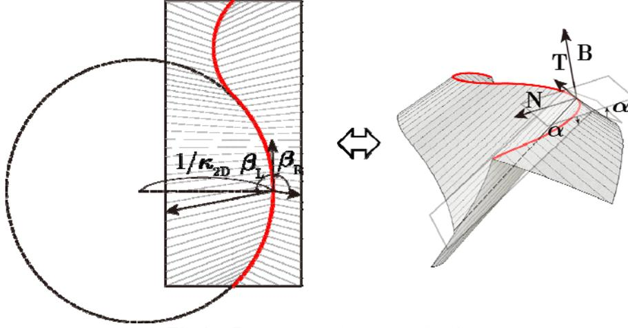
Fig.1 : Parameter of curved folding.
