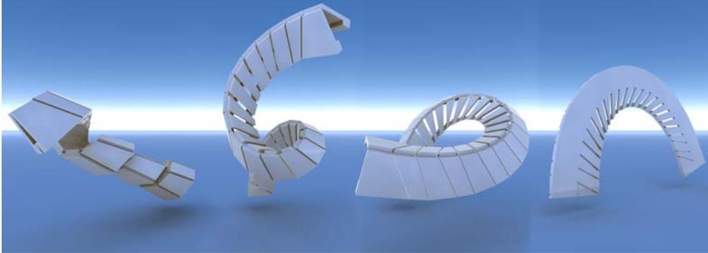
*Fig. 5: Folding sequence of the structure from single curve. Solid model based on thick panel construction technique [5].*
