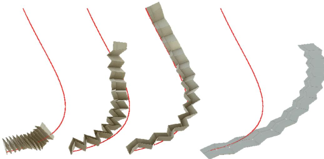
*Fig. 7: Folding sequence of the zig-zagged structure. The folded form approximates the original space curve drawn in red.*
