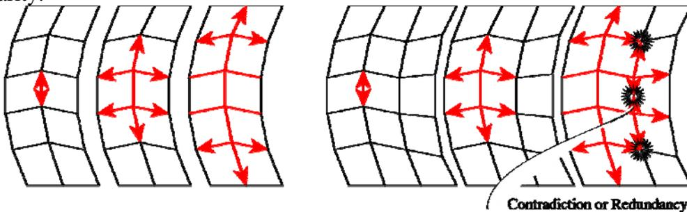
Fig. 4: One-DOF foldable mechanism (left) vs. over constrained mechanism (right).
