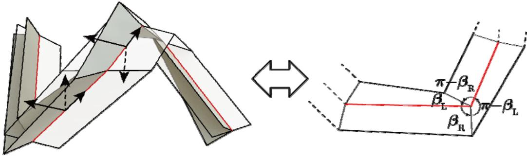
Fig. 3: Discrete curved folding with constant folding angle..Note that every vertex is flat-foldable in the isometric sense, i.e., Kawasaki's theorem is satisfied (alternating sum of incident angles is 0).
