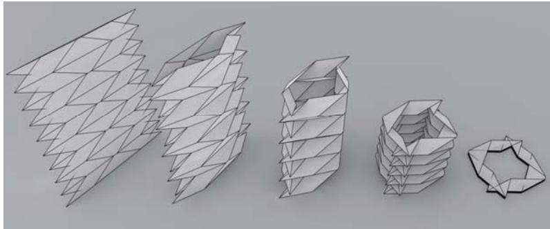
Fig. 9: The cylinder of  $\alpha=30^\circ$  at  $\beta = 89^\circ, 67.5^\circ, 45^\circ, 22.5^\circ, 1^\circ$  (from left to right).
