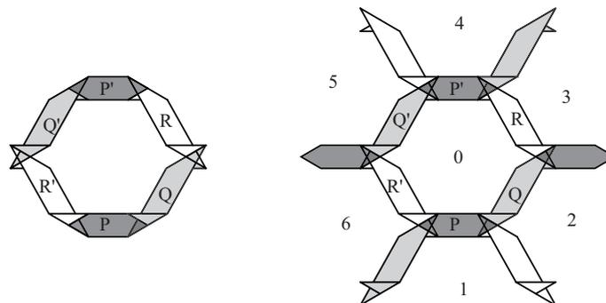
Fig. 16: Correspondence of parts to adjacent cylinders. Parts  $\{P, P', Q, Q', R, R'\}$  of cylinder 0 is shared by adjacent cylinders  $\{1, 4, 2, 5, 3, 6\}$ , respectively.
