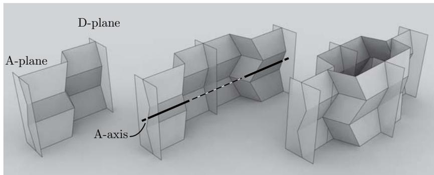
Fig 7: Symmetry operation to construct a cylinder by composing the modules.
