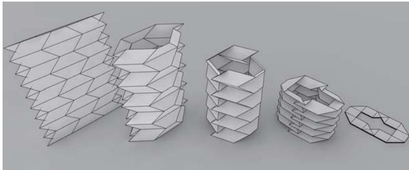
Fig. 10: The cylinder of  $\alpha=45^\circ$  at  $\beta = 89^\circ, 67.5^\circ, 45^\circ, 22.5^\circ, 1^\circ$  (from left to right).
