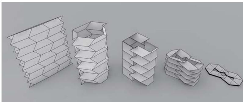
Fig. 11: The cylinder of  $\alpha=54^\circ$  at  $\beta = 89^\circ, 67.5^\circ, 45^\circ, 22.5^\circ, 1^\circ$  (from left to right).
