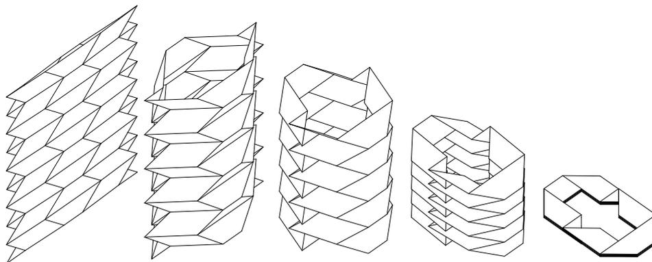
Fig.3: Star-polyhedron with a synchronized motion.
