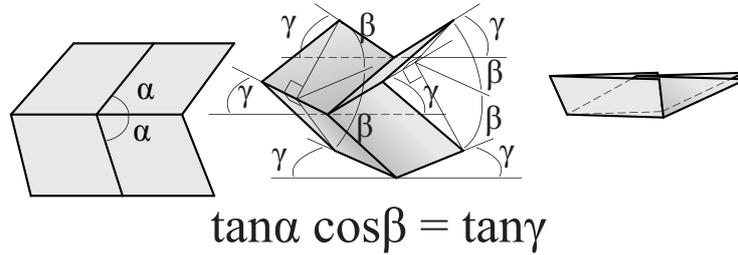
$\alpha$  = constant: an inner angle of parallelogram
