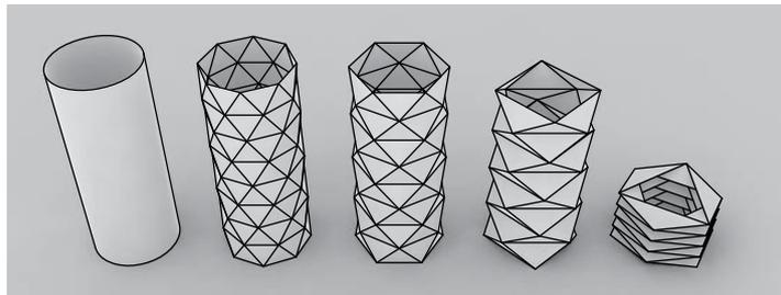
Fig.1: Yoshimura Patterns. From Left to Right: Original cylinder and Yoshimura Patterns of radial frequency of 8, 6, 4, and 3. Note that each state is static.
