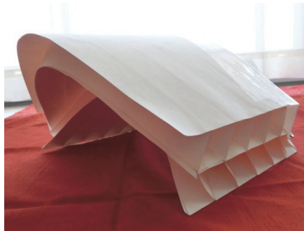
Figure 8. Model of deployable vault structure.
