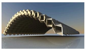
Movie S4. Folding sequence of an architectural canopy structure created from geometrically varied zipper-coupled tubes.
