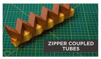
Movie S1. Zipper-coupled tubes. Shown are assembly from two single tubes, flat folding, eigenmodes, and system actuation from one end.
