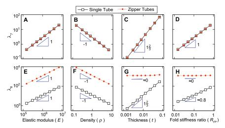
Fig. S4. Eigenvalue sensitivity for a single tube and the zipper-coupled tubes. (A–D) Scaling of  $\lambda_7$  with respect to E,  $\rho$ , t, and  $R_{FP}$ . (E–H) Scaling of  $\lambda_8$  for the same cases. These relations directly govern the scaling sensitivity of the bandgap.
