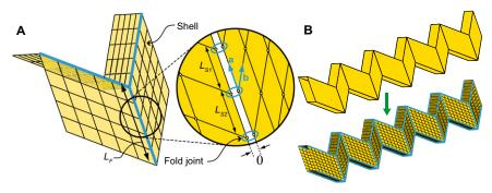
Fig. S5. FE model used for verification. (A) Miura-ori cell discretized with D = 5 elements for each panel; *Inset* shows local zero-length connectivity at fold lines. (B) Discretization of single tube with D = 8.
