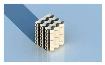
Movie S3. Folding sequence of a cellular origami metamaterial consisting of zipper and aligned tubes.
