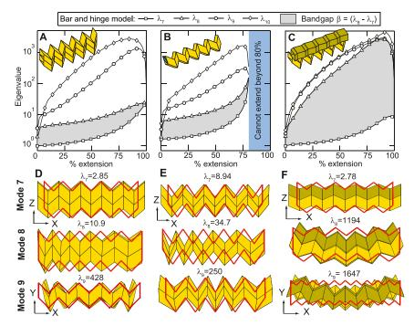
Fig. S8. Eigenvalue comparison for the different coupling assemblies. (A–C) Eigenvalue vs. extension for the aligned-, internally, and zipper-coupled structures, respectively. (D–F) Seventh, eighth, and ninth deformation eigenmodes when structures are at 70% of the maximum extension length (undeformed outline in red).
