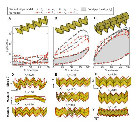
Fig. 56. Eigenvalue analyses of a sheet, a single tube, and a zipper-coupled tube performed with the FE model. (A–C) Eigenvalue vs. extension for the three structures, performed with both the FE and the bar and hinge models. (D–F) Seventh, eighth, and ninth deformation eigenmodes when structures are at 70% extension (undeformed outline in red).
