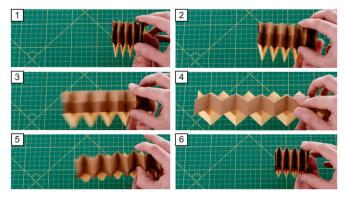
**Fig. 1.** Deployment and retraction sequence of a zipper-coupled tube system. This origami has only one flexible motion through which it can deform, and thus it is deployed by actuating only on the right end. See Movie S1 for complete simulation.
