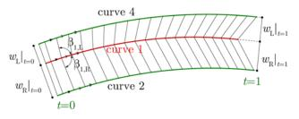
Fig. 03. Construction of curves 2 and 4, indicating the change in the proportion.
