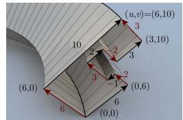
Fig. 06. Derived curve is defined by two parameters u and v (the sequence does not matter).
