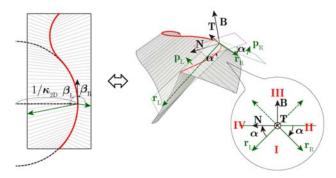
Fig. 02. Parameters (Left: Crease pattern, Right: Folded form in perspective and orthogonal projection along vector **T**.
