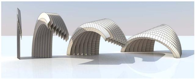
Fig. 09. Folding motion of an example vault constructed form foldable tubes.
