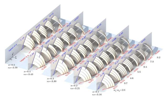
Fig. 10. Variations of the derived form; the slope of the section in the zx plane is indicated in blue and the slope in the xy plane is indicated in red.
